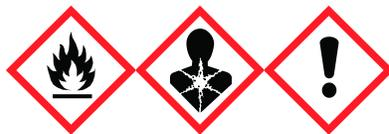
**Signal word** Danger**Hazard statement** Flammable liquid and vapor. Causes skin irritation. Causes serious eye irritation. May cause respiratory irritation. Causes damage to organs through prolonged or repeated exposure.**Precautionary statement****Prevention**
